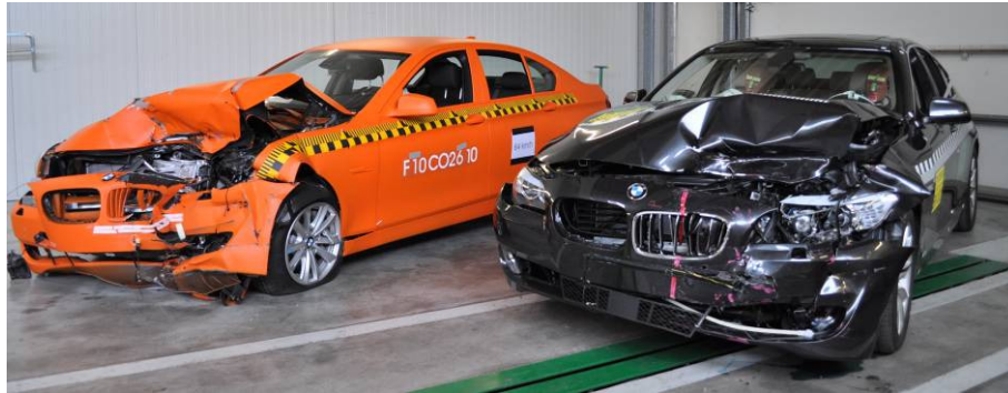
Figure 9. Comparison of the deformation of the front of the two test vehicles
