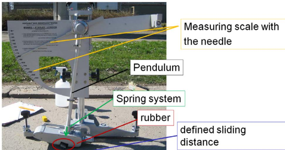
Picture 2: construction of the SRT - pendulum
