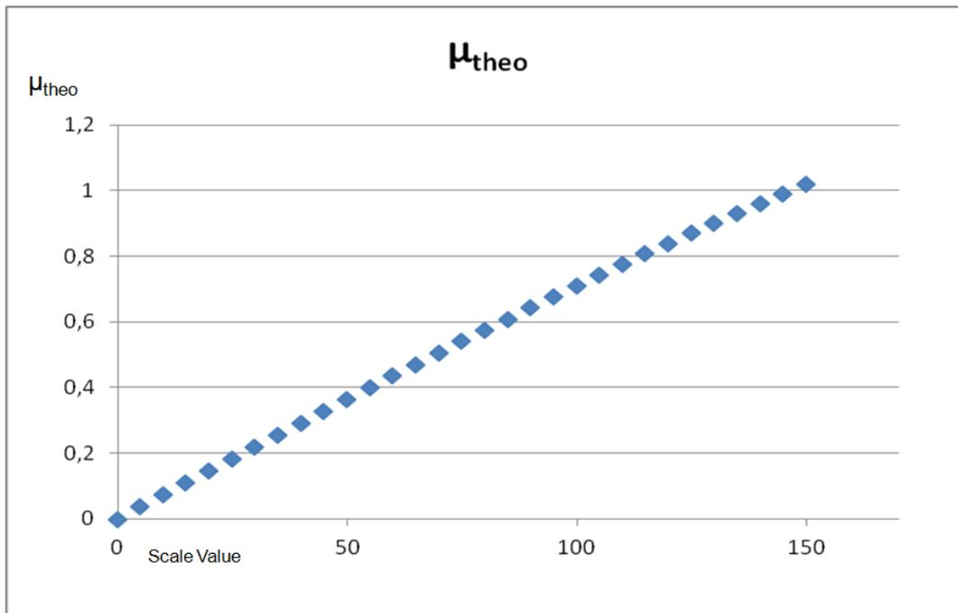
Figure 1: theoretical friction coefficient in dependence of the SRT - scale value
