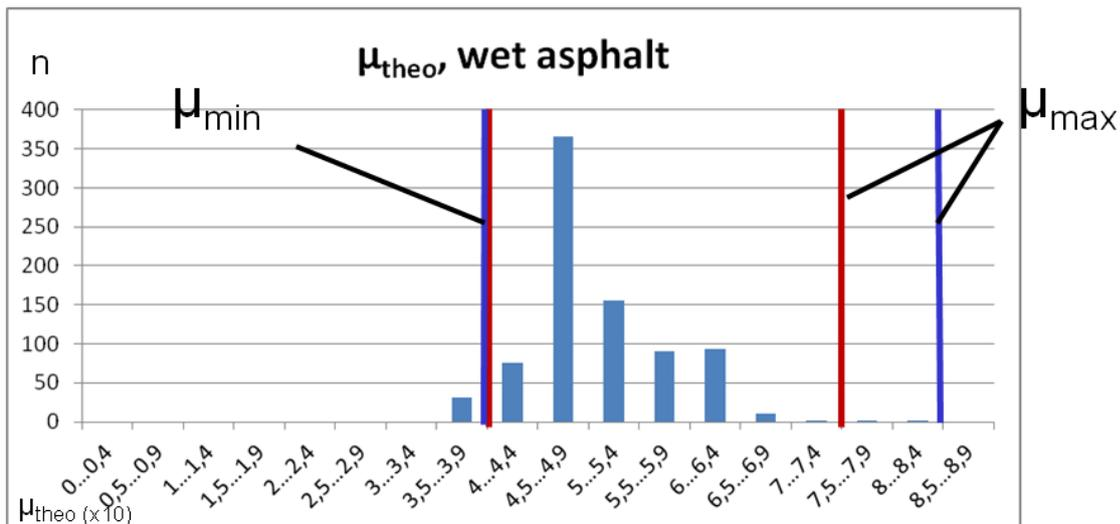
Figure 3: Theoretical friction coefficient calculated out of the measured SRT-values in comparison to applied decelerations
