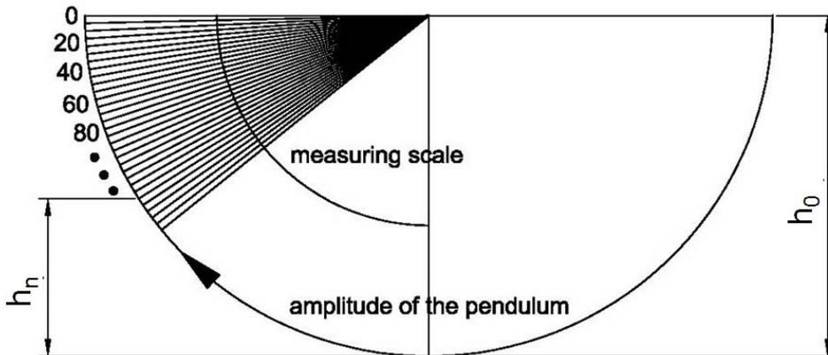
Figure 6: principle of the pendulum process
