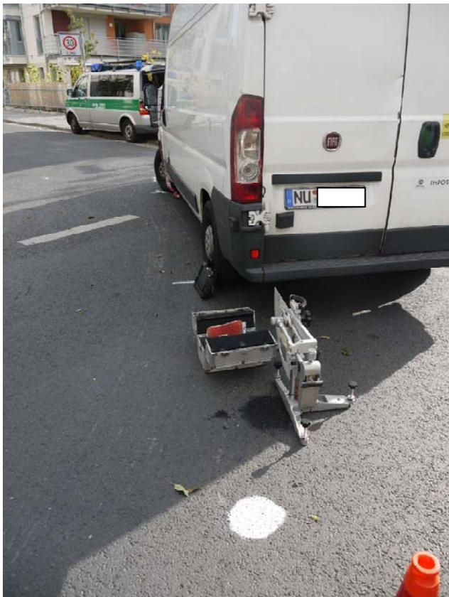
Picture 1: measurement of the micro- and macroroughness at the accident site
