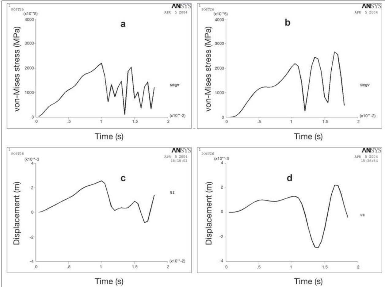
**Fig. 4:** Von-Mises stress plot and displacement (in the direction of impact) plot with impact duration for pelvis without car door and padding (a and c respectively) (from MAJUMDER et al. [11]) and for pelvis with car door and padding (b and d respectively) (present study), analyzed by ASIS® software
