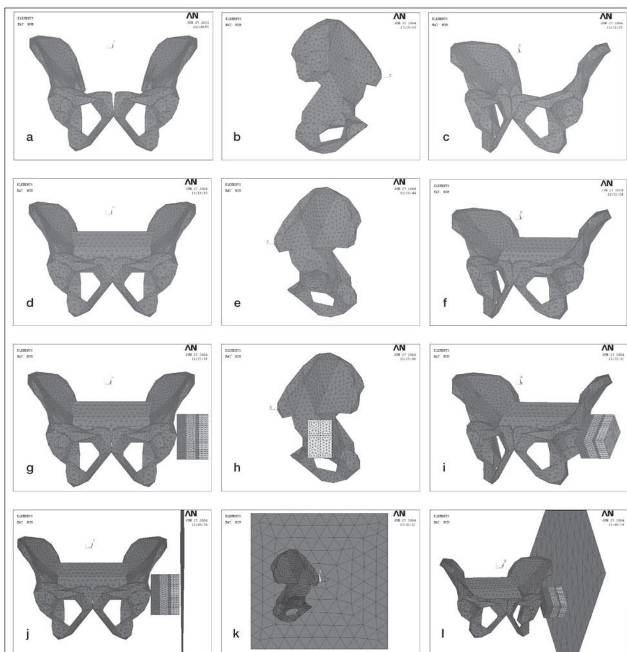
**Fig. 1:** Different views of the three-dimensional finite element models, (a-c): Only pelvis without sacrum, from MAJUMDER et al. [10]; (d-f): Full pelvis with idealized sacrum for this study and from MAJUMDER et al. [11]; (g-i): Full pelvis with equivalent car door structure; (j-l): Rigid wall with which full pelvis with equivalent car door structure collided
