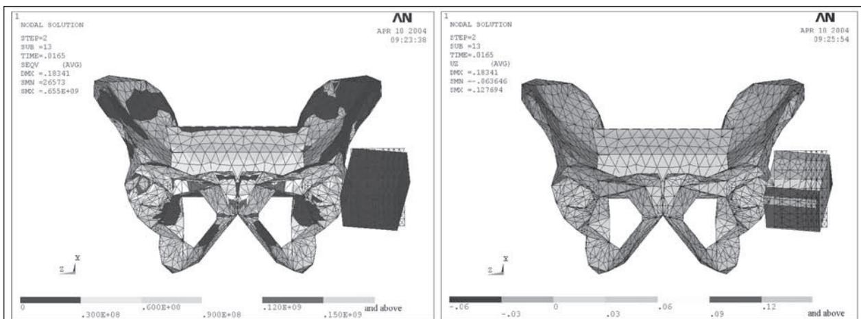
**Fig. 5:** (a) von-Mises stress (MPa) and (b) displacement (m) contour in the direction of impact, for the pelvis with car door structure and padding, at 16.5ms, for the first load case, analyzed with ANSYS® software
