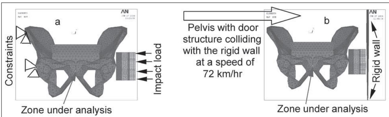
**Fig. 3:** Impact load cases for analysis with (a) ANSYS<sup>®</sup>, (b) ANSYS-LS-DYNA<sup>®</sup> software
