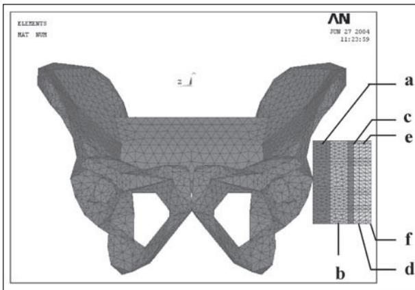
**Fig. 2:** Three-dimensional finite element model (22,967 tetrahedral and 5,820 shell elements through 5,824 nodes) of human pelvis with layers of soft tissue and equivalent car door structure (a – Soft tissue; b – Styrodur<sup>®</sup> Foam; c – Plastic (UHMWPE); d – Steel; e – Glass; f – Steel)
