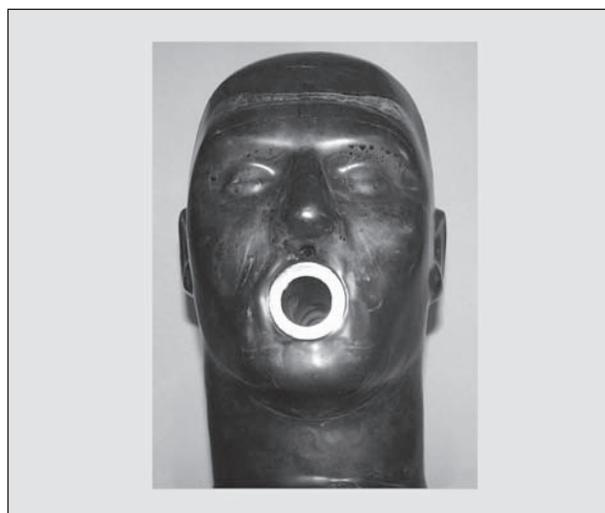
**Fig. 1:** Headform used to measure CO<sub>2</sub> concentrations. Barely discernible is a hole to which the gas detector tube was connected, between nose and mouth opening
