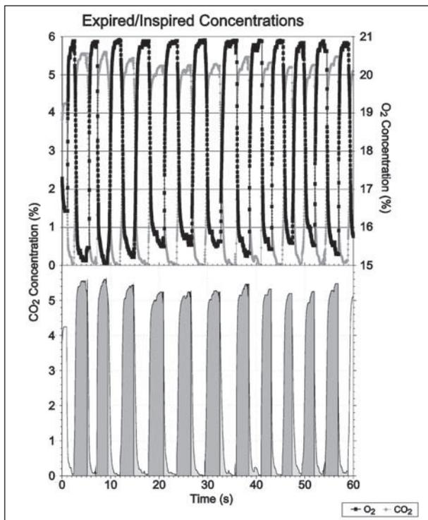
**Fig. 3:** Upper: Time-dependent concentrations of the indicated gases at the mouth of a subject wearing an integral helmet with visor closed and zero wind. Lower: The  $\text{CO}_2$  concentration analyzed for exhalation and inhalation portions of the breathing cycle, as described in the text
