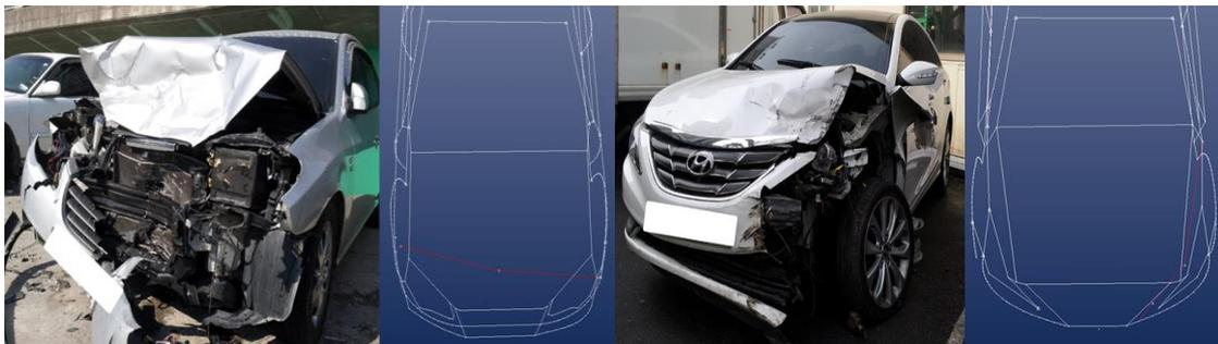
Figure 9. Vehicle deformations calculation using PhotoModeler
