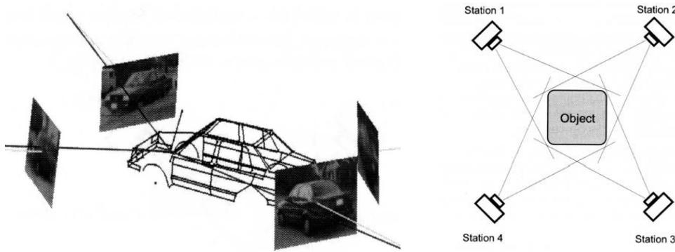
Figure 9. Application of photographic technique (from PhotoModeler Manual)
