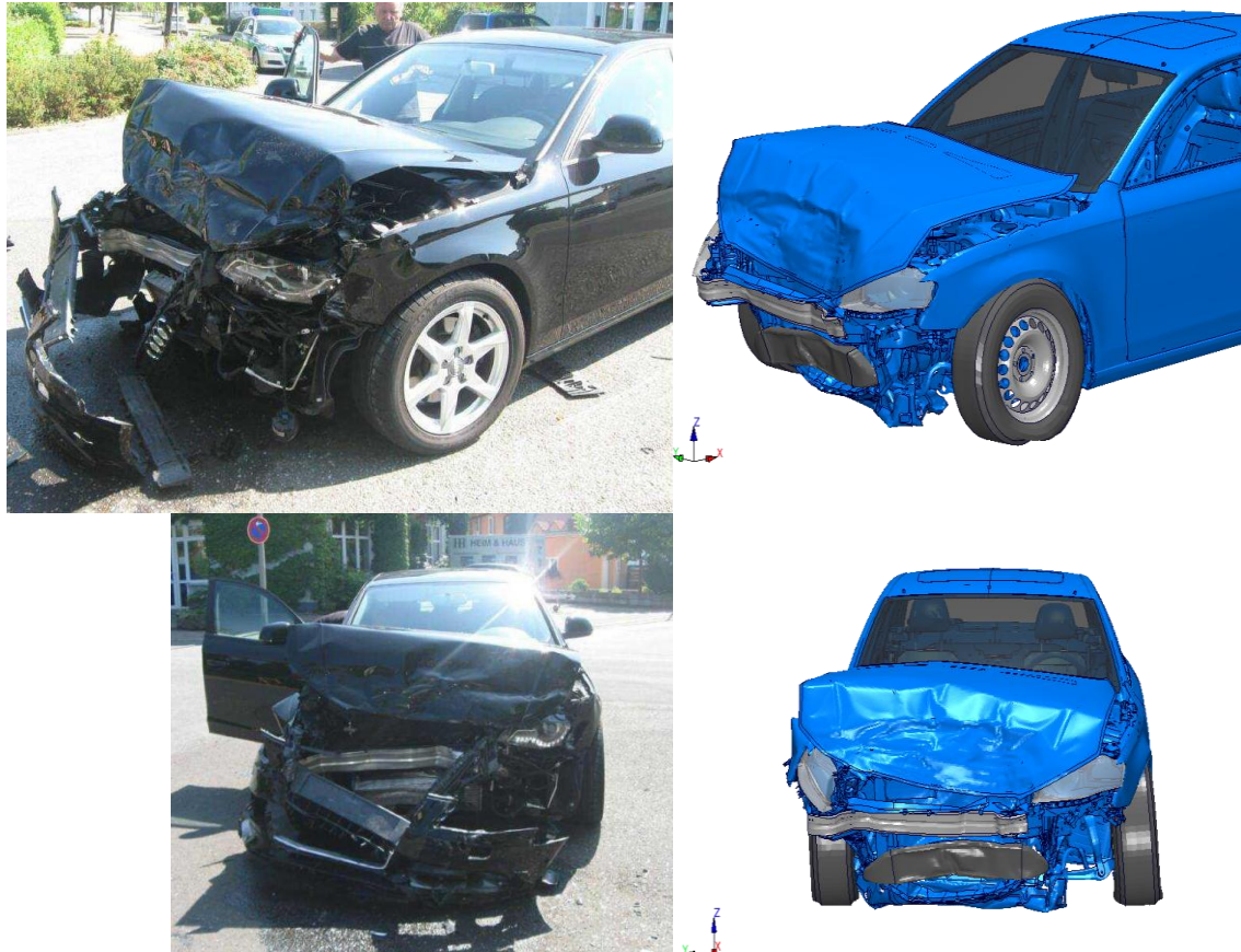
Figure 5. Structure deformation comparison. Right: Real accident. Left: Simulation. Credits: Adrian Langner.
