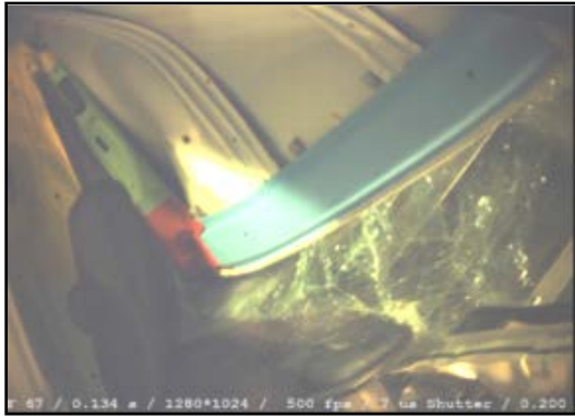
Video Still of Production Cab Deformation (35.5 in (90.2 cm) of A-pillar Displacement)
