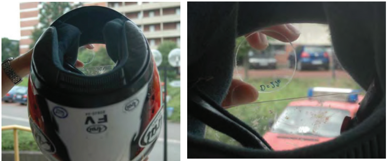
Figure 3. There are 6 different reference discs L with light transmittance values of \tau = 14\% , 57\% , 64\% , 81\% , 83\% and 91\% . There are also 4 different reference discs with light diffusion values of D = 2\% , 8\% , 16\% and 25\% .
