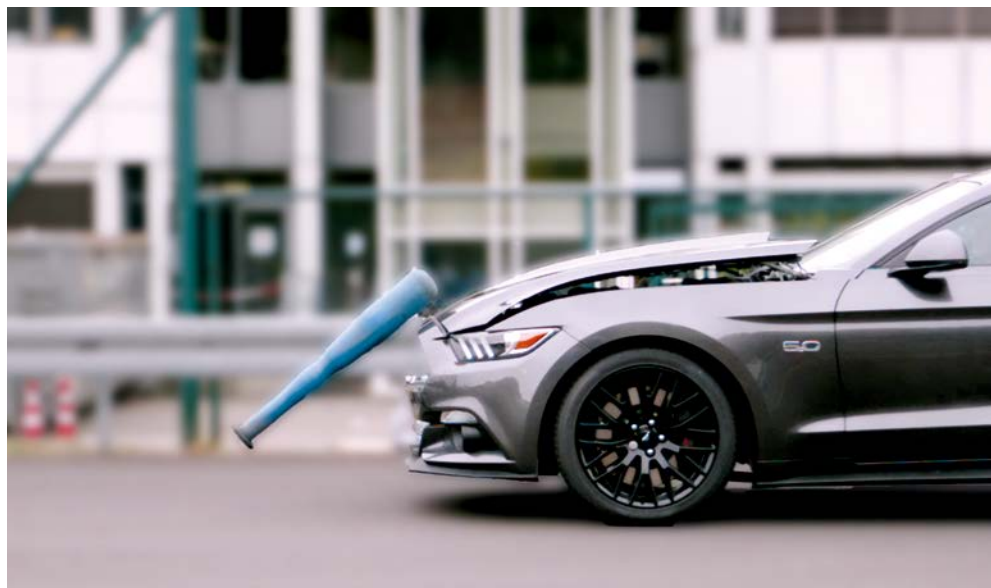
Testing the sensors of an active systems in an impact test against a pedestrian surrogate.
