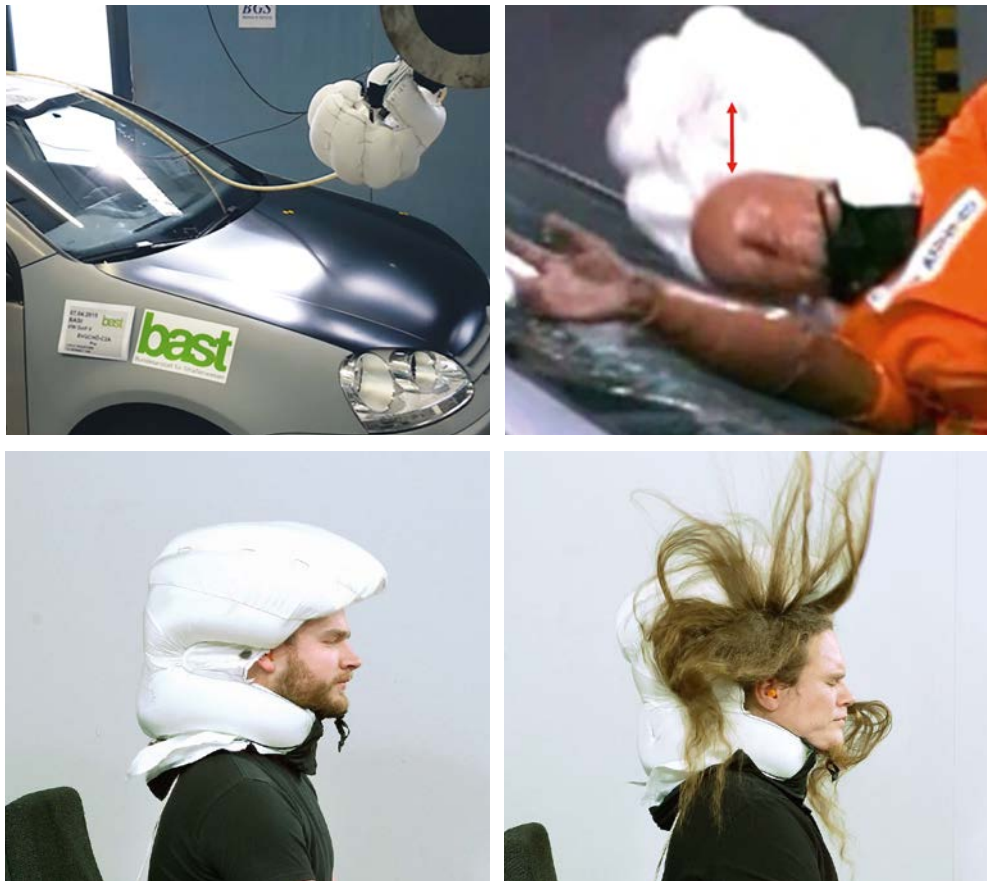
Component tests on bonnet (top left); head impact on passenger car front at insufficient positioning of the airbag (top right); airbag inflation in short hairstyles (bottom left); airbag inflation in long hairstyle (bottom right).
