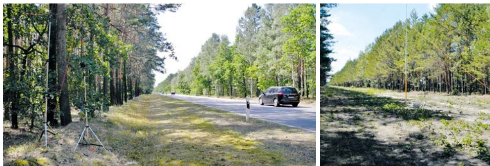
Acoustic measurements at a forest strip along the rural road B97 near Hoyerswerda.
