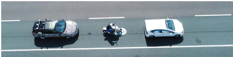
Sample test scenario "motorcycle at the tail end of a traffic jam".
