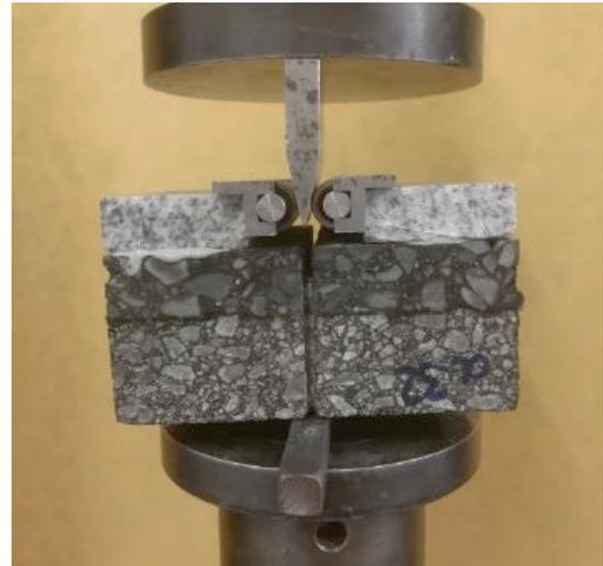
Figure 3: test device for monotonic wedge opening tests
