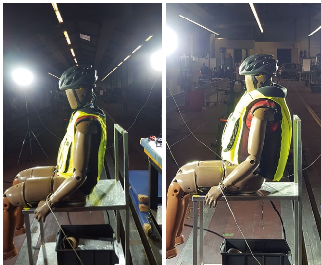
Airbag vest in stationary test: undeployed and deployed
