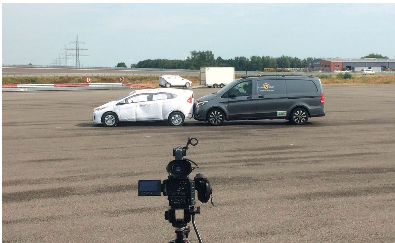
Testing the emergency braking assistance system to prevent or mitigate rear-end collisions
