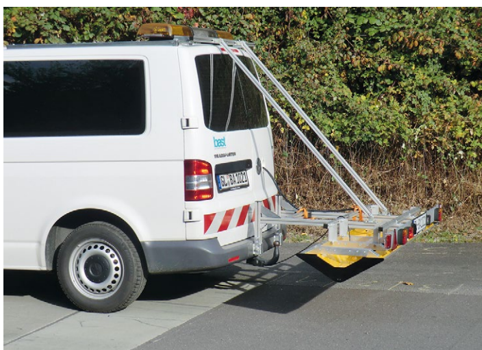
BAST's 3D georadar system in operation
