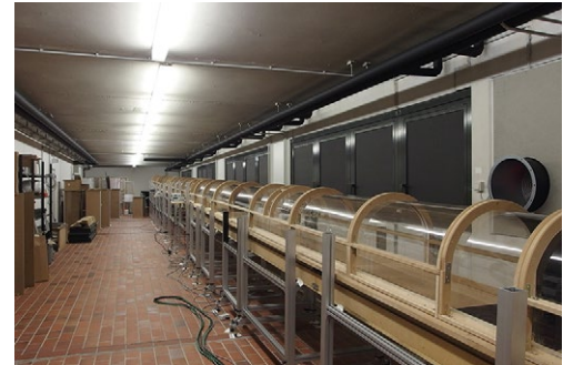
Simulation of large-scale fire tests in the model tunnel
