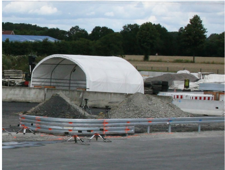
Sketch of a curved safety barrier for junctions (left) and prototype on a test field (right)
