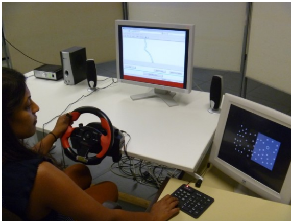
Figure 2: Experimental set-up for a triple-task scenario which combines visual tracking task, SuRT and TDRT
