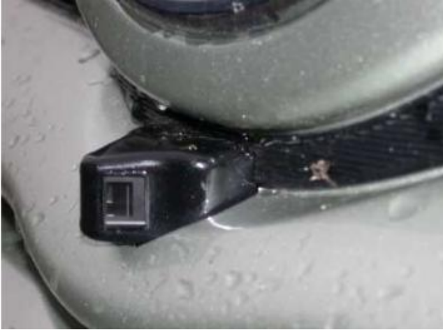
Figure 4: One-camera-system, integrated in the emblem of the car
