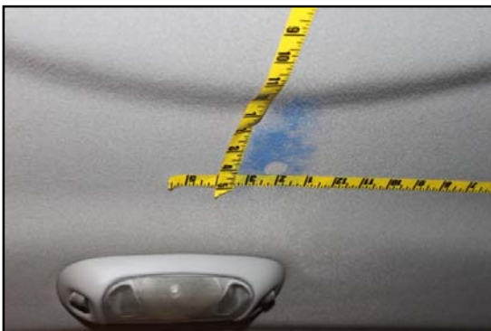
Figure 12. Post Test Damage, Test 5b – Roof Panel Impact
