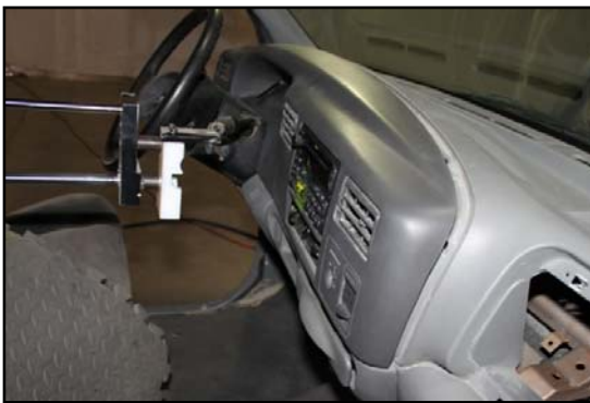
Figure 11. Post Test Damage, Test 5c – Dash Impact
