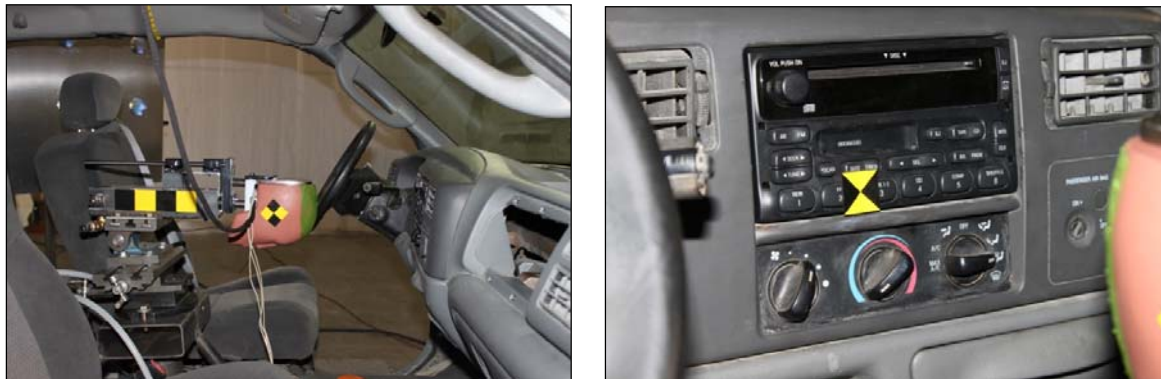
Figure 8. Series 5 Test Setup For Horizontal Impact Into Dash Radio
