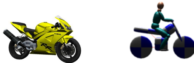
Figure 7. Model of motorcycle without rider and multibody models of motorcycle and rider.
