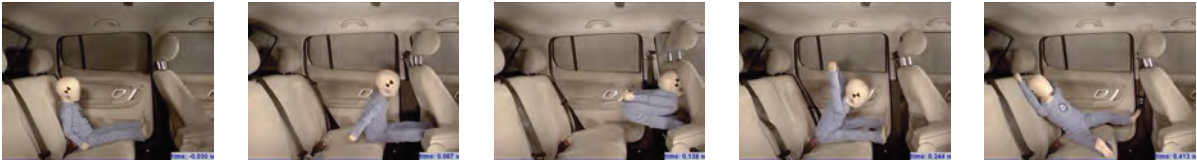
Figure 2 Frontal crash test – child without use of child restraint system protection
