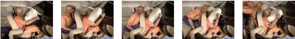
Figure 3 Frontal crash test – unrestrained rear passenger is killing the driver after impact
