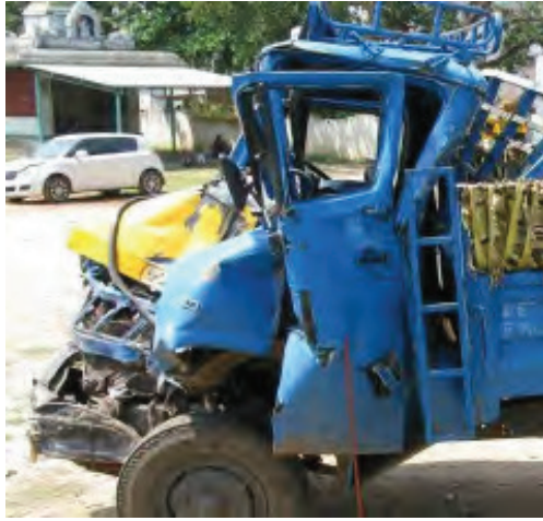
Figure 10. Intrusion Measurements of a Truck Colliding with Roadside Tree
