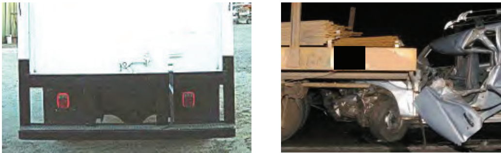
Figure 7. UPD in a Truck (left) and an Under-Ride Crash (right)
