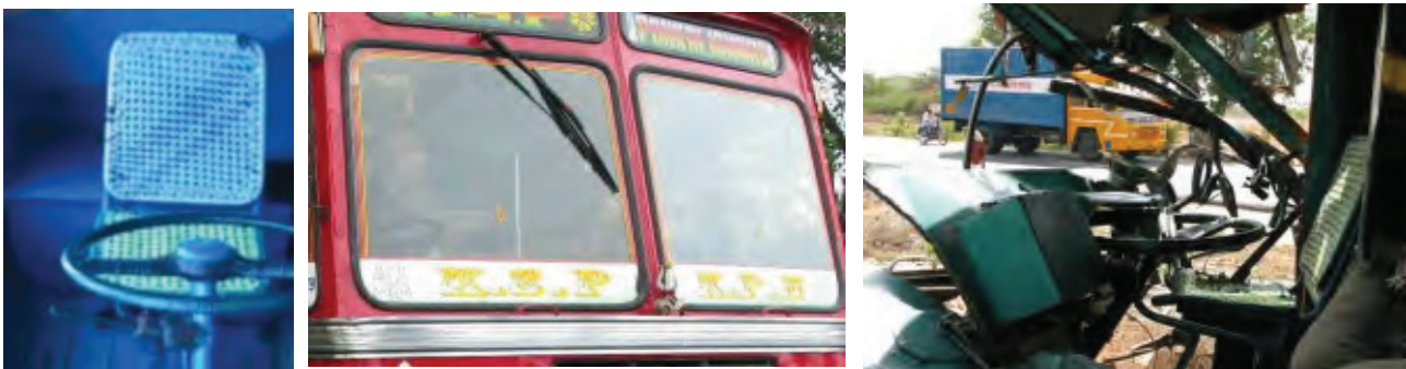
Figure 9. Poor Seating for Truck Drivers and Absence of Seat Belts (left); Wiper Availability only on Driver Side (center); Weak Cab Strength (right)
