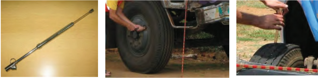
Figure 6. Truck Tire Pressure Gauge (left), Researcher Checking Tire Pressure (center), Tread Depth of Crash Involved Truck (right)
