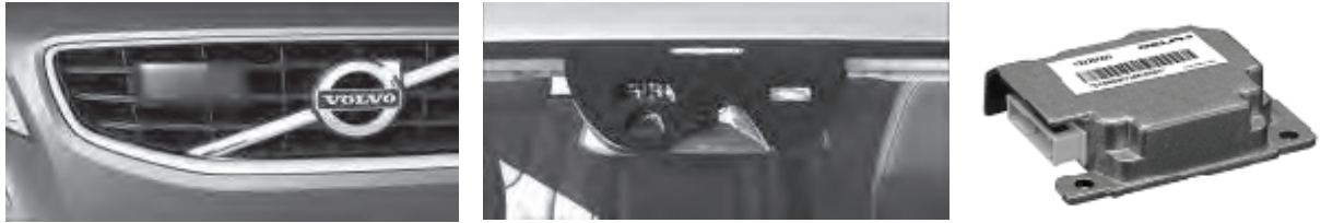
Figure 5. From left: Electronic Scanning Radar (FLR) in the grille, Forward Looking Camera (FLC) mounted behind windscreen and the Forward Sensing Module (FSM) control unit.
