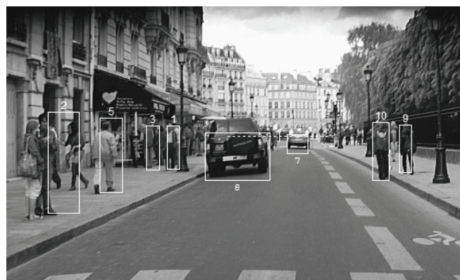
Figure 4. Visualization of how pedestrians are detected in Collision Warning with Full Auto Brake and Pedestrian Detection (CWAB-PD).
