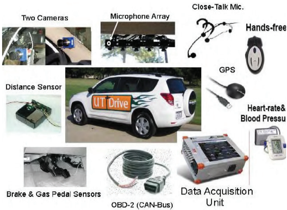
Figure 1. Data collection vehicle and incorporated sensors
