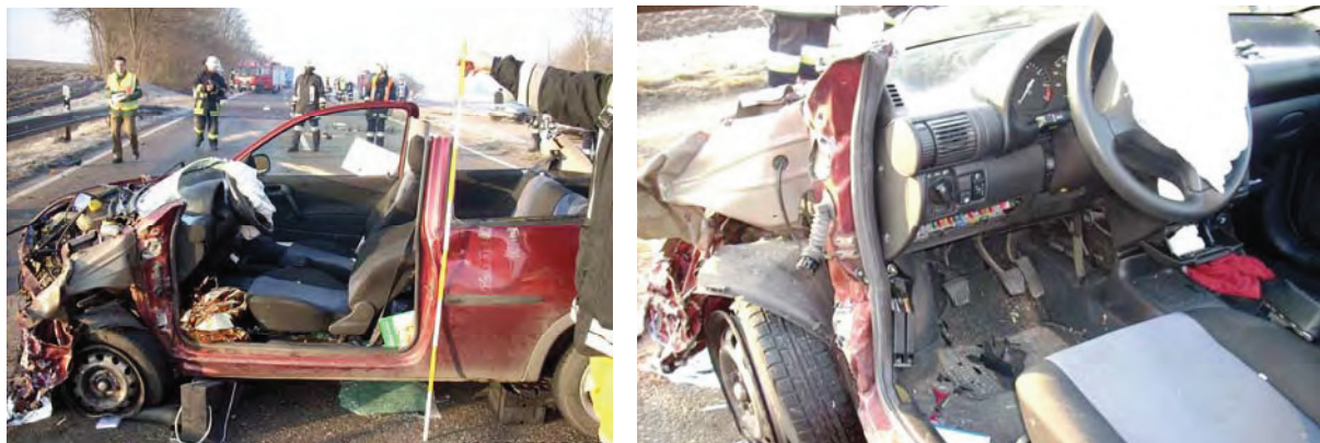
Figure 5. Example of documentation by fire department using yard stick for reference (source: Kreisbrandinspektion Günzburg)
