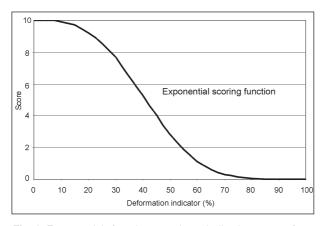
Fig. 2: Exponential function used to built the score from relative deformation
