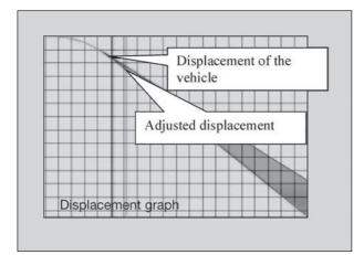
The effect of extension or reduction of the plateau length in terms of speed and displacement is calculated and visualised. The right adjustment value is reached when the effect on displacement corresponds to the difference of average deformations between the accidented and the tested vehicle.
