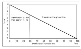
Fig. 1: Linear function giving the score as a function of absolute deformation
