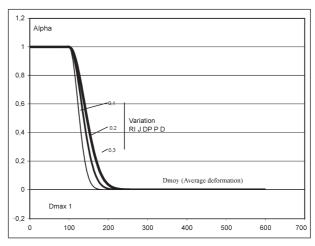
Fig. 3: Variation of coefficient  $\alpha$  as a function of the average of the deformations measured on the real world vehicle and on the reconstruction vehicle. D<sub>lim</sub> and  $\gamma_1$  condition the shape of the curve
