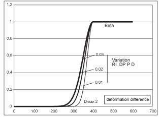
Fig. 4: Variation of coefficient  $\beta$  as a function of the relative difference of deformations measured on the real world vehicle and on the reconstruction vehicle. E<sub>lim</sub> and  $\gamma_2$  condition the shape of the curve
