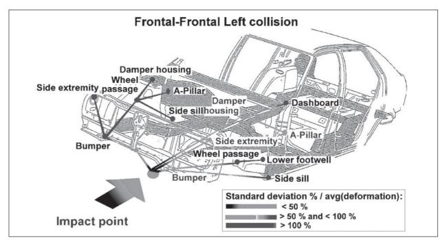
Fig. 6: Variability of deformations measured at various locations of the vehicle structure
