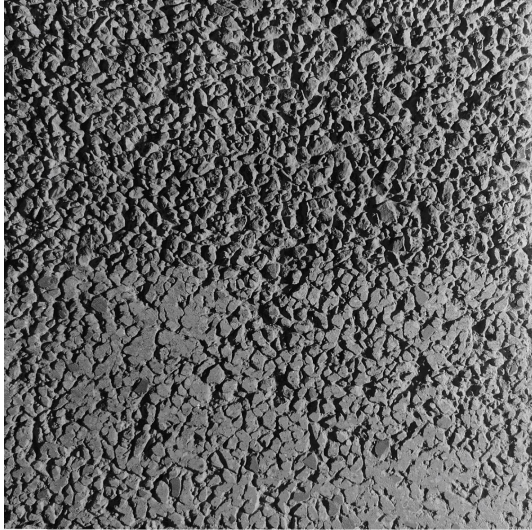
Fig. 8: Laboratory slab with the lower half grinded and an overall more even texture
