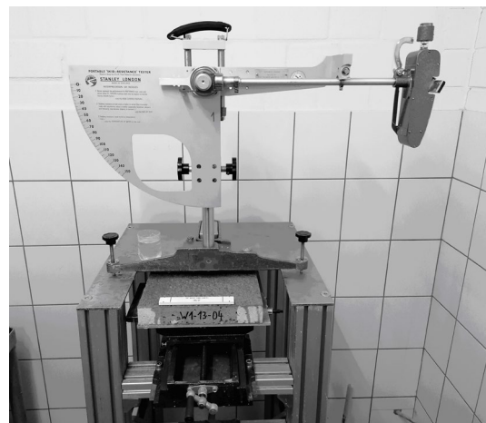
Fig. 4: Test table for SRT measurement of the slabs with shifting device for the concrete slabs
