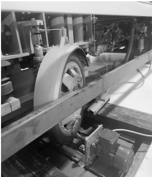
Fig. 9: Measuring vehicle with SKM measuring mechanics on the roller test bench.
