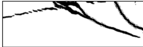
T18_DIC_S - Querkraft: 462.0 kN
