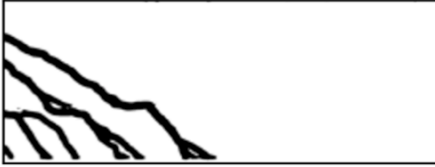
T18_DIC_F - Querkraft: 289.0 kN
