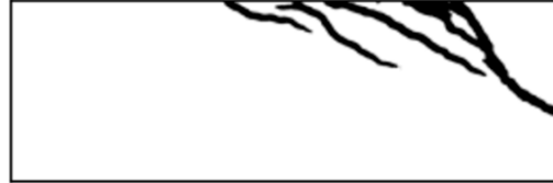
T22_DIC_S - Querkraft: 365.0 kN
