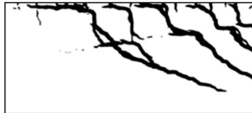
R22_DIC_S - Querkraft: 413.0 kN
