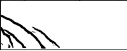
T22_DIC_F - Querkraft: 304.0 kN
