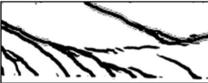
T22_DIC_F - Querkraft: 547.0 kN
