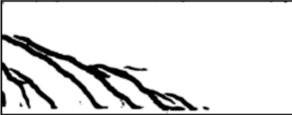
T22_DIC_F - Querkraft: 426.0 kN
