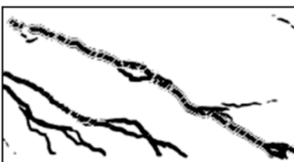
R25_DIC_F - Querkraft: 483.0 kN
