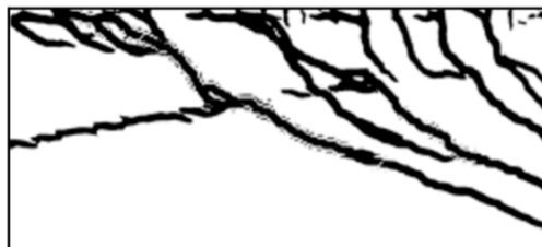
R18_DIC_S - Querkraft: 584.0 kN
