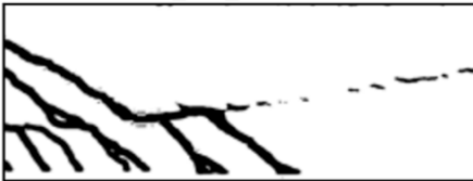
T18_DIC_F - Querkraft: 405.0 kN
