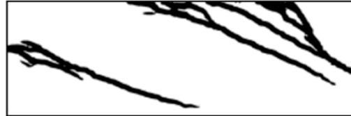
T22_DIC_S - Querkraft: 487.0 kN
