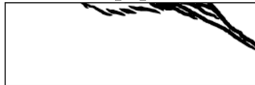
TG25_DIC_S - Querkraft: 525.0 kN
