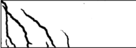
DLT25_DIC_F - Querkraft: 335.0 kN
