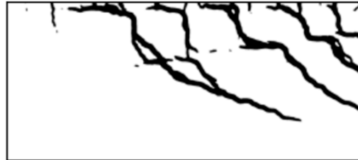
R22_DIC_S - Querkraft: 311.0 kN
