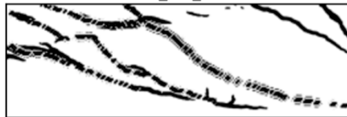
T25_DIC_S - Querkraft: 510.0 kN
