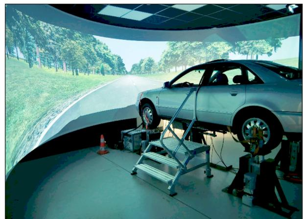
Fig. 2: The driving simulator
