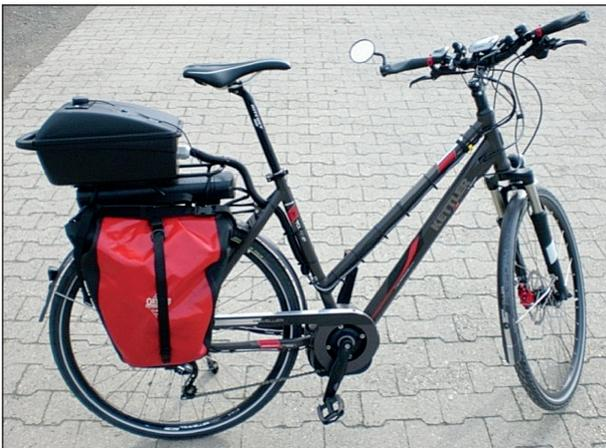
Fig. 2 : Electric bike with permanently installed measuring devices
