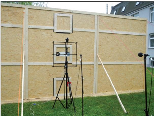
Fig. 5.1: Setup for measurements at test noise barrier with geometrical exact leakages
