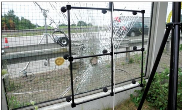
Fig. 5.5: Test setup for measurement of transmission loss of noise barrier with defect in situ
