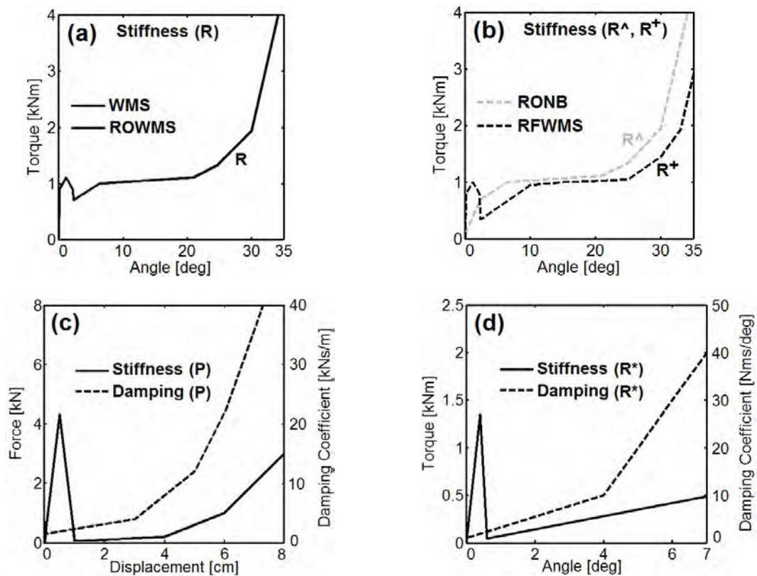
Figure 4. The mechanical properties of the car-seat models
