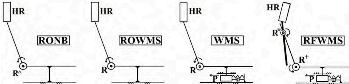
Figure 3. The car-seat models used in head-restraint evaluation
