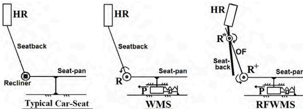
Figure 2. Schematic drawings of car-seat models
