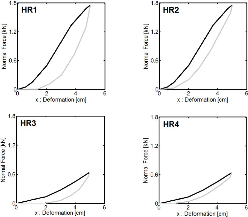
Figure 6. The mechanical properties of the head-restraints HR1, HR2, HR3, HR4
