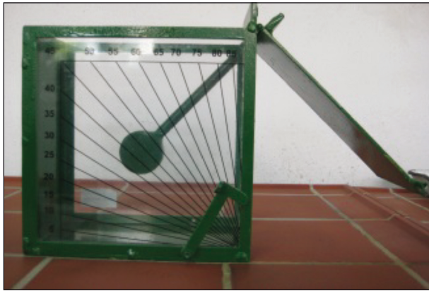
Fig. 1: Flow box according to SONNTAG
