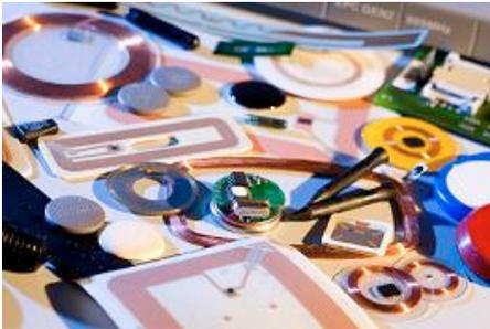
**Abb. 11:** RFID-Chips (<http://www.rfid-webshop.com>)
