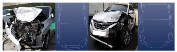
Figure 9. Vehicle deformations calculation using PhotoModeler
