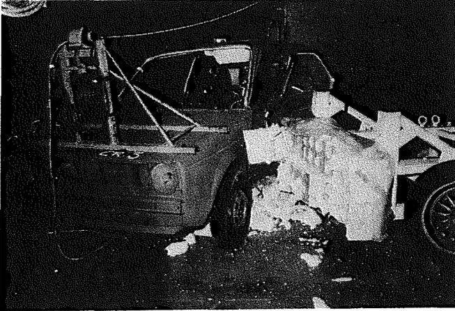
Fig. 8: Rest position after a collision with the "crabbed" EEVC barrier
