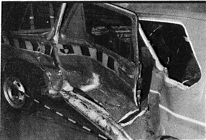
Fig. 6: Lateral deformation of the moving VW Golf after being struck by a DB W 123
