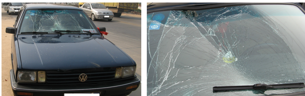
Fig.2. The head impact location on the windscreen of the car in adult bicyclist accident
