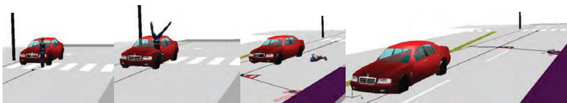
Figure 7. Car-to-pedestrian (1) real accident simulated on PC-Crash ®
