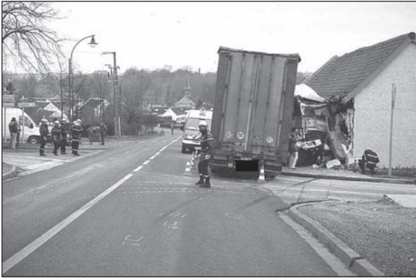
Fig. 4: Vehicle marks on the road and rest position of the vehicle
