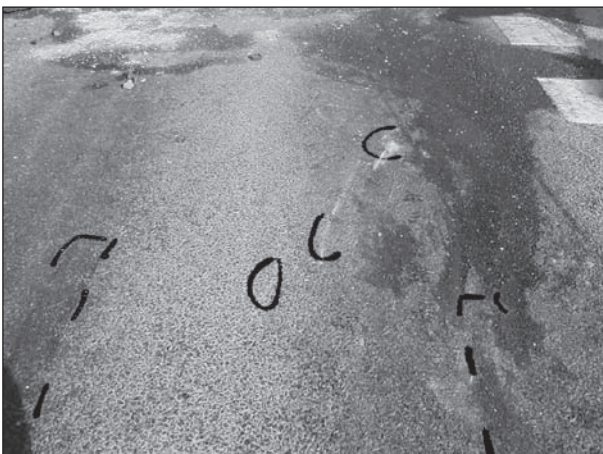
Fig. 6: Scratching marks, point of impact
